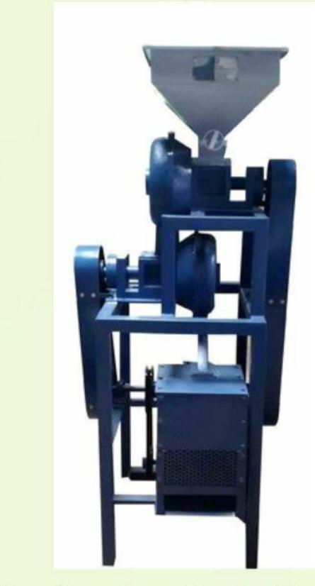
Double chamber De-huller
