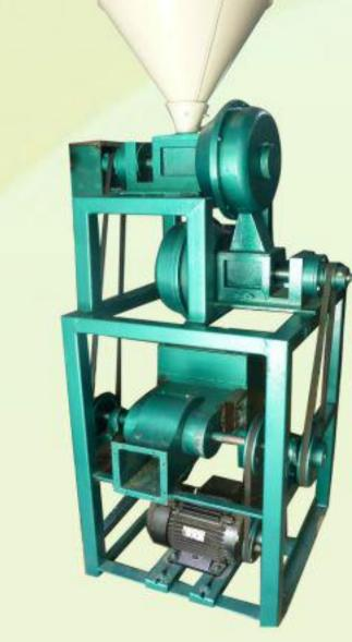
Double chamber De-huller
